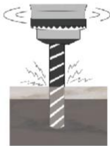
Drill hole in the ground Ø: 19mm Depth:40mm
