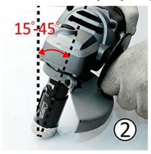
3. Bring the drill up into upright position, Continue to drill and swaying the machine along a circle.
