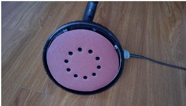
Remove the sandpaper, put the Allen wrench into the hexagon hole in the center of the viscid disc and then rotate clockwise to take off the damaged viscid disc. Install the new viscid disc (see the picture).
