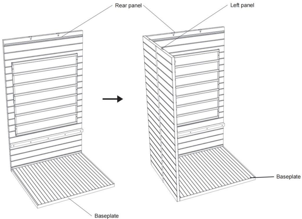
Take out the rear panel and left panel stand it at the corresponding position behind the base plate.
