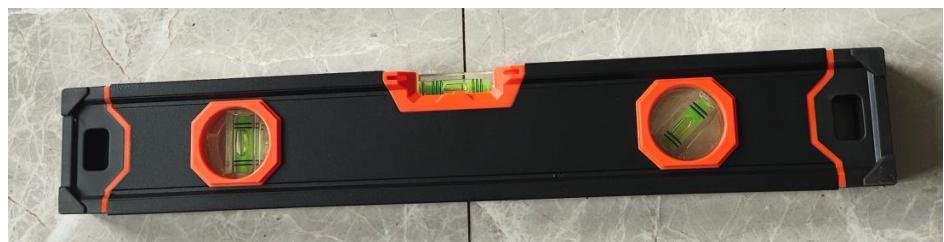
The 24-inch bubble level is 600mm long, with measurable angles of 0 ,45 and 90 degrees. If you buy the model SP-C4 or SP-C6, the bottom working face is magnetic, and the rest of the models are not magnetic.
