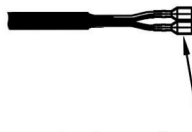
Connector type of seat safety switch: 40C
