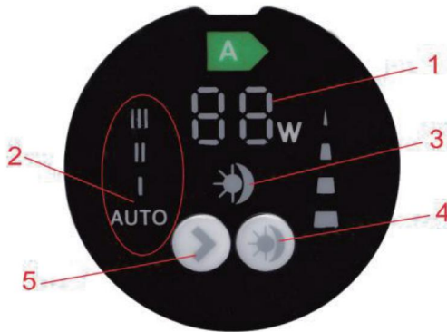
Figure 7 THE CONTROL PANEL
