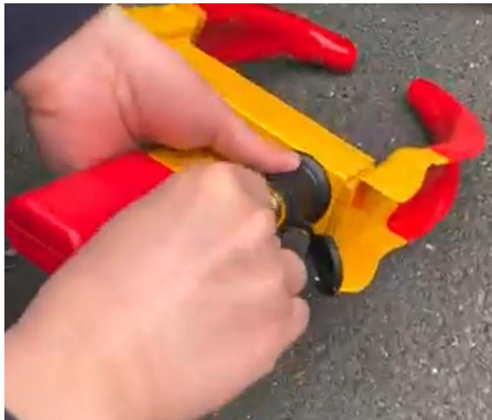
Step1:Use the key to open the lock
