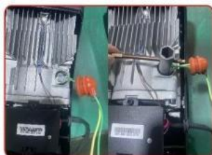
Step3 The third step is to open the buckle cap, Remove ignition plug with special wrench
