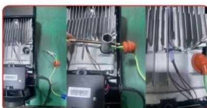
Step4 Replace the new ignition plug Fasten the buckle cap
