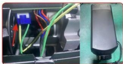
Step3 The third step is to open the buckle cap, Remove ignition plug with special wrench
