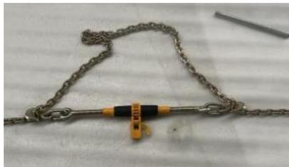
3. Set the switch to LOWER, insert the handle into the handle hole, and turn the handle clockwise back and forth to tighten the chain; Set the switch to upper and turn the handle counterclockwise back and forth to release the chain. And then remove the handle, as shown in the picture.
