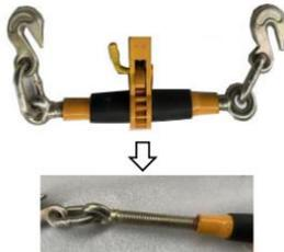
2. Pull the chain tight manually, then hook the chain with the binder, as shown in the picture.
