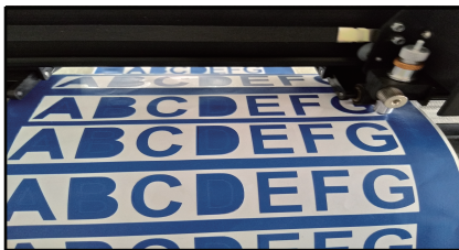
The output is completed, the cutting plotter is cutting. pic 5-10
