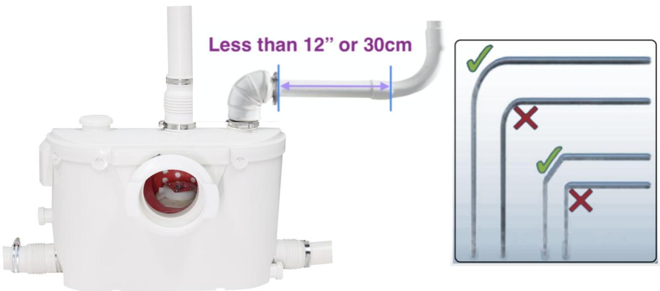
Then incline 2%-3% to lead the water drainage pipe to main pipeline, otherwise, the sewage will return flow. Additionally, the elbow position of PVC water pipe must use 135° big elbow, but not 90° elbow, otherwise, it will affect the range.
