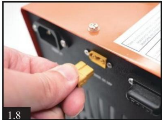
Using DC I2V Car Battery Power
