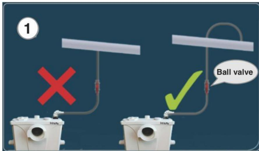
(5-6), For best performance, please drain upward first and then drain the drain pipe to the main pipe at a 2%-3% incline: otherwise, the sewage will flow back.
