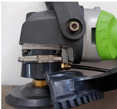
3. Install the grinding plate and select the appropriate polishing pad.
