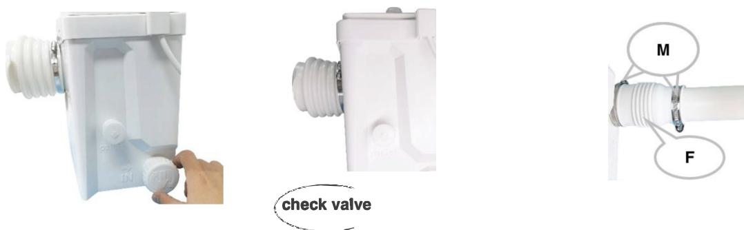
The pipe size for connecting the shower or washbasin wastewater to the pump is 40mm. If connecting the shower, the bottom of the shower needs to be raised by 20cm, and the drain pipe must maintain a 3 % slope to let the wastewater flow into the pump by gravity, preventing the wastewater from staying in the inlet pipe and producing an odor. If not connecting a toilet, use accessory (G) to plug the water inlet at the front of the pump. Refer to the following installation diagram:
