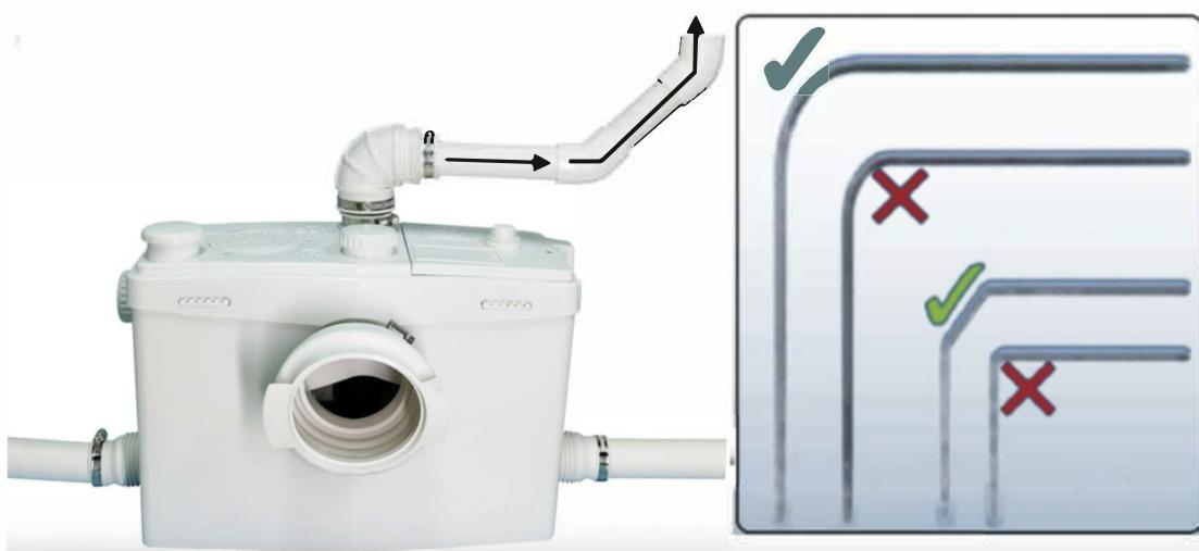
The schematic diagram of the drain pipe installed on the side is:
