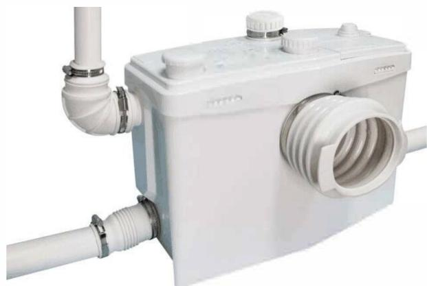
Note: To achieve the best performance of the pump, first drain upwards, then horizontally. When draining horizontally, the drain pipe should have a downward slope of 10-15 degrees. Do not use right-angle (90 degrees) elbows, as they will affect the vertical lifting effect.
