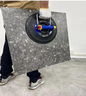
4. After complete inflation, check the red warning line to see if it has retracted. If it has not retracted, then the object can be moved.
