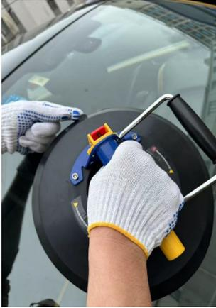
5. After the transportation process is completed, gently lift the deflation tongue or press the black deflation button to remove the suction cup.
