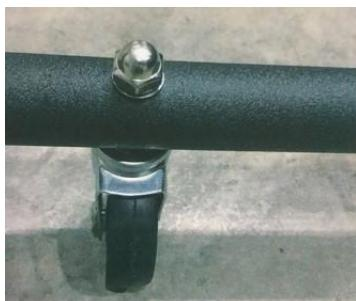
8. Attach the lock washer and acorn nut to each caster.
