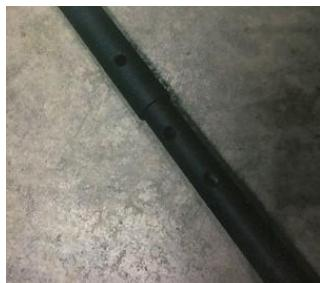
6. Line up the holes as shown, according to your vehicle's year. (Align the outside holes for Wranglers. Holes for JK 07 - 17)
