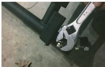
10. Tighten each lock washer and acorn nut using a crescent wrench.
