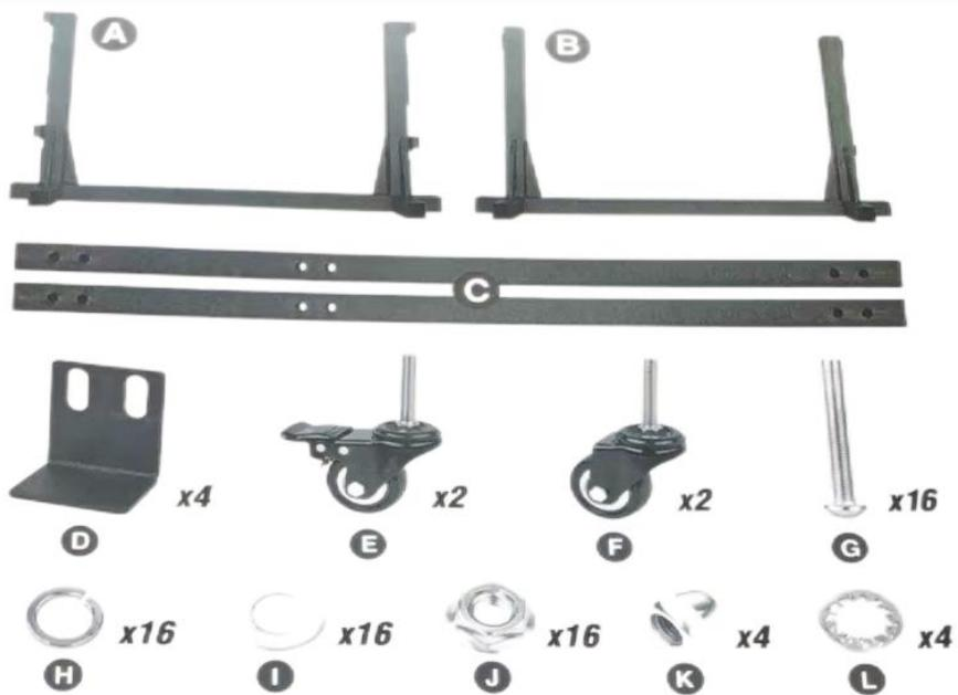
1. Connect the parts "A", "B" and "C" together in the following way (The hole circled near part "B").
