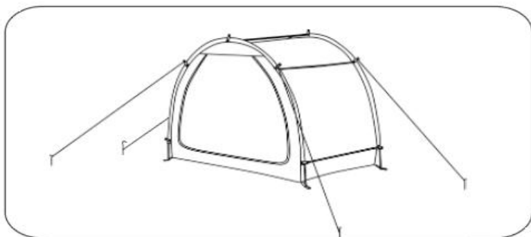
STEP-5: Fixed wind rope ground nail
