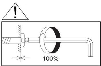
After installing all the parts according to the illustration, tighten the screws
