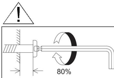
Install the corresponding parts according to the connecting lines in the drawing. When installing, pay attention to the screws on one side not to tighten, reserve a gap to facilitate the next step of installation
