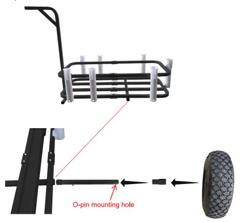
**NOTE:** Insert the axle into the ends of the bottom cross member of the frame, then insert the plastic parts of the axle, and finally install the wheel.
