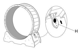
\* H wooden lock isinserted into the card slot and locked.
