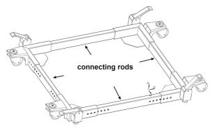
**Note**: To ensure the connection strength, the connection position needs to be fixed with two bolts, not only one.
