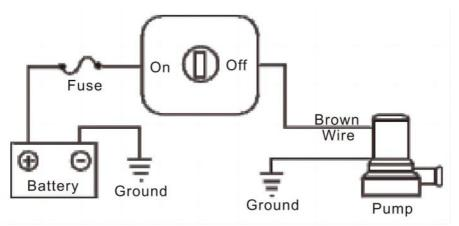
Wiring for Automatic Operation
