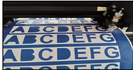
The output is completed, the cutting plotter is cutting. pic 5-10
