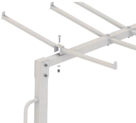
Place first chair hook on crossbar (3). Align hooks hole with crossbar (3) hole. Insert crossbar retaining screw T4 (1 for each). Tighten screw with nut cap using metal key. Repeat all the other hooks.
