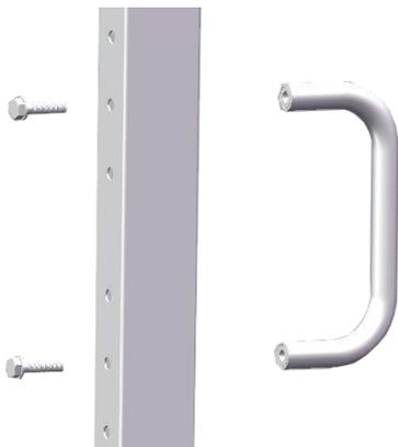
Finally, attach your side handle. Choose a height setting. Place handle on vertical bar. Insert retaining screws T2 (2 for each handle). Tighten screws using the hex key. Repeat for the second handle.
