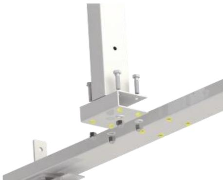
Take vertical bar (1) and place it in the middle of the bar(2). Make sure the rail part of the bar faces in. Insert retaining screws T3 (4 for each bar). Tighten screws with nut cap using wrench keys. Repeat for the other side.
