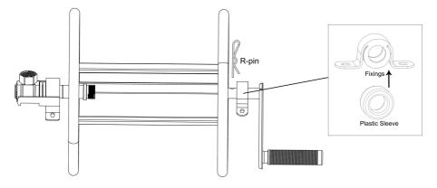
2. Fix the hose reel to frame 2 with M6\*40 Bolt & M6 Look Nut & M6 washer.
