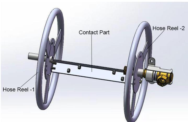
2. Put part 4 (Plastic Sleeve) into part 2 ( Fixings), then put part 2 on part 3 (Hose Reel-1).
