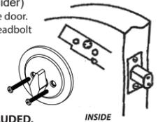
Attach the inner trim with a 25"(64mm) machine and tighten it securely.
