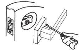
Attach the inner knob with 1" (25 mm) or 1.5" (39 mm) screws at 12:00 and 6:00 o'clock.
