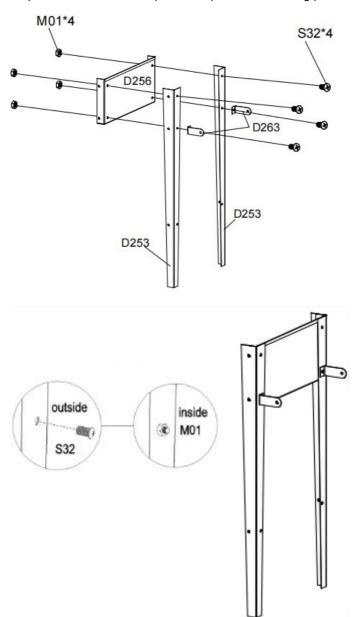
Step2: Install the foot, hook, side plate, and axle of the other end.
