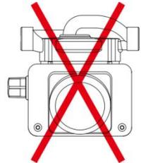
The pump must keep the rotor shaft installed horizontally
