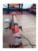
7. The height of the knife frame is 3mm higher than the center line of the main shaft and the tail seat. The height of the knife frame varies with the diameter of the cutting wood. Generally speaking, the larger the diameter of the wood, the higher the height of the knife, the smaller the diameter of the wood and the lower the height of the knife frame.
