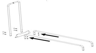
3. Connect one L-shaped frame and 2pcs of U-shaped connectors tube to the already assembled part and fasten with 4pcs M8\*60m screws and nuts. As the picture shows:
