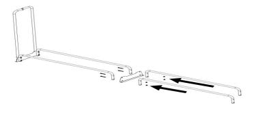
4. Assemble another side frame with the completed part of step 3, then fasten with 4pcs M8\*60m screws and nuts. As the picture shows:
