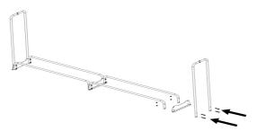
5. After assembly is completed, the L-shaped connection pad is fixed with expansion screws in the middle to increase the stability of the rack. The holes on the side of the connection pad are pre-drilled and can be fixed freely as required. As the picture shows:
