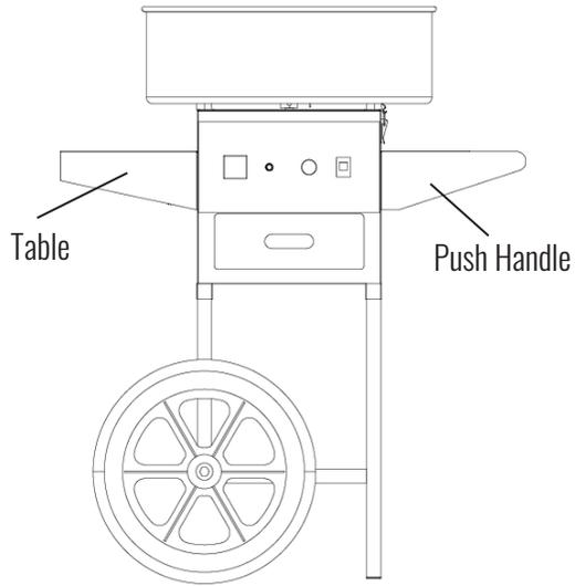
4. Place the stainless steel pan on top of the box and fix it with the 4 locking clips on both sides.
