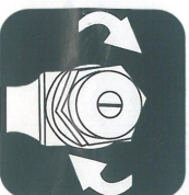
Reinstall the nozzle and keep the groove level with the rotary rod
