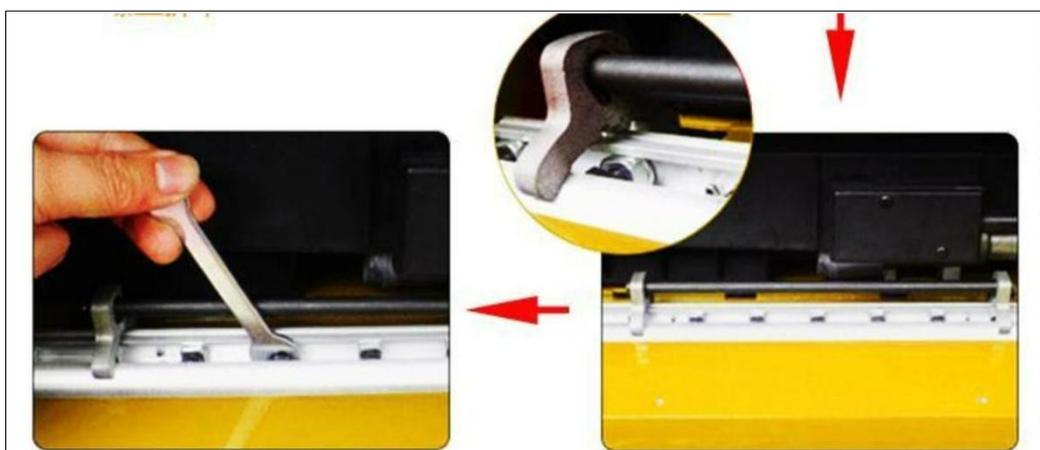
**Warning!** Check that total 18 screws are tightened. Turn the blade holder by hand to check that it rotates easily and smoothly.
