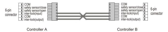
Note: Two doors share same sensor or same signal source, both doors may hold open, in this case, exchange two signal wires of the sensor which is connected with the same controller, it doesn't matter controller A or B.
