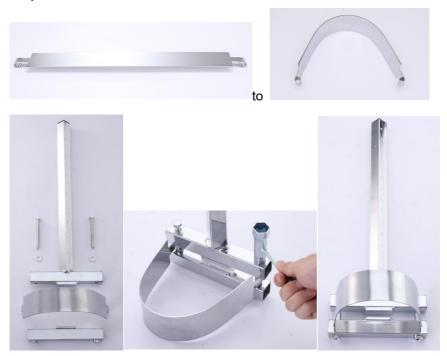
Insert two M8x75 bolts (item#19)through adjustment post(item#5). Slide bolts through nose guard (item #11) and through clamping braket(item#6). Start hex head bolts(item#19) into nuts on bottom of braket. leave loose so there is a gap for mounting chainsaw bar!
