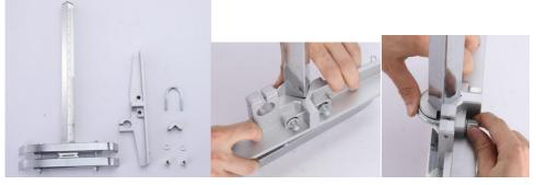
Attach thrust and post assembly t end bracket using U-clamp (item#12) post camp (item#13) two i washer (item#18),and coupling nuts(item#17).
