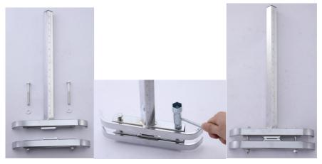
Insert two M8x75 bolts (item#19) through adjustment post (item#1) and into clamping bracket(make sure the side of the adjustment post with measurements on it is facing away from you when assembling)(item#2)engaging nuts on bottom of clamping braket. leave loose so there is a gap for the saw bar!
