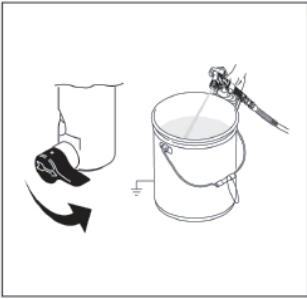
11、 Close relief valve. Flushing pail gun trigger to discharge fluid hose.
