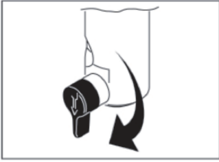
9、 The filler valve downward rotation.
