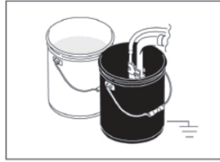
10、 The siphon tube set into the inner fluid filled with grounded metal pail. Pull to the wire with the bucket connected to a true earth ground. The oil is stored in sprayer washed away. Rinse water-based paint, oil paint and storage oil rinse with mineral spirits.
