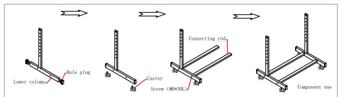
Please insert the Hole plug to the Lower column. Spin the wheel into the fixed lower column and secure the two connecting rods in the lower column with the screws of the  $M6 \times 30$ . Get component one
