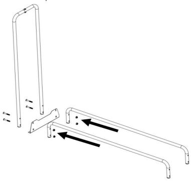
3. Please install another side frame with the same way, and connected with base frame by 4pcs M8\*60mm screws. As the picture shows:
