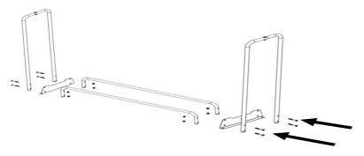
4. After assembly is completed, the L-shaped connection pad is fixed with expansion screws in the middle to increase the stability of the rack. The holes on the side of the connection pad are pre-drilled and can be fixed freely as required. As the picture shows:
