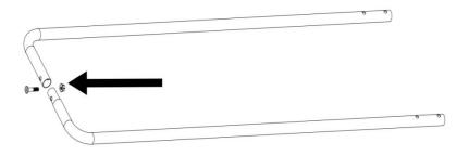
2. Please install the U connector with the side frame, and screw on with the pad by 4pcs M8\*60mm screws. As the picture shows:
