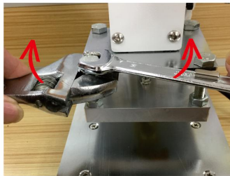
●Hot stamping plate balance adjustment: first loosen the screws in reverse direction with the wrench, when the screw adjustment in clockwise direction, hot stamping plate is up, otherwise is down.
