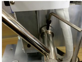
●Stroke control fixed ring: fixed Stroke in order to control the depth of hot stamping.(Digital specific)
