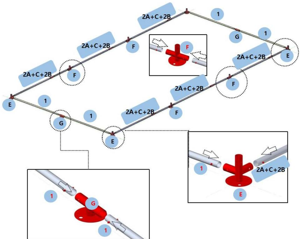
**Step3:** Install the column according to the part number below.
