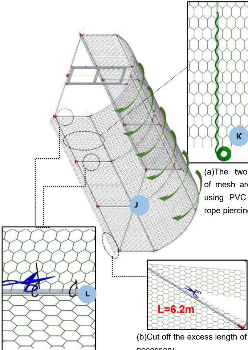
(a) The two pieces of mesh are joined using PVC lashing rope piercings.
