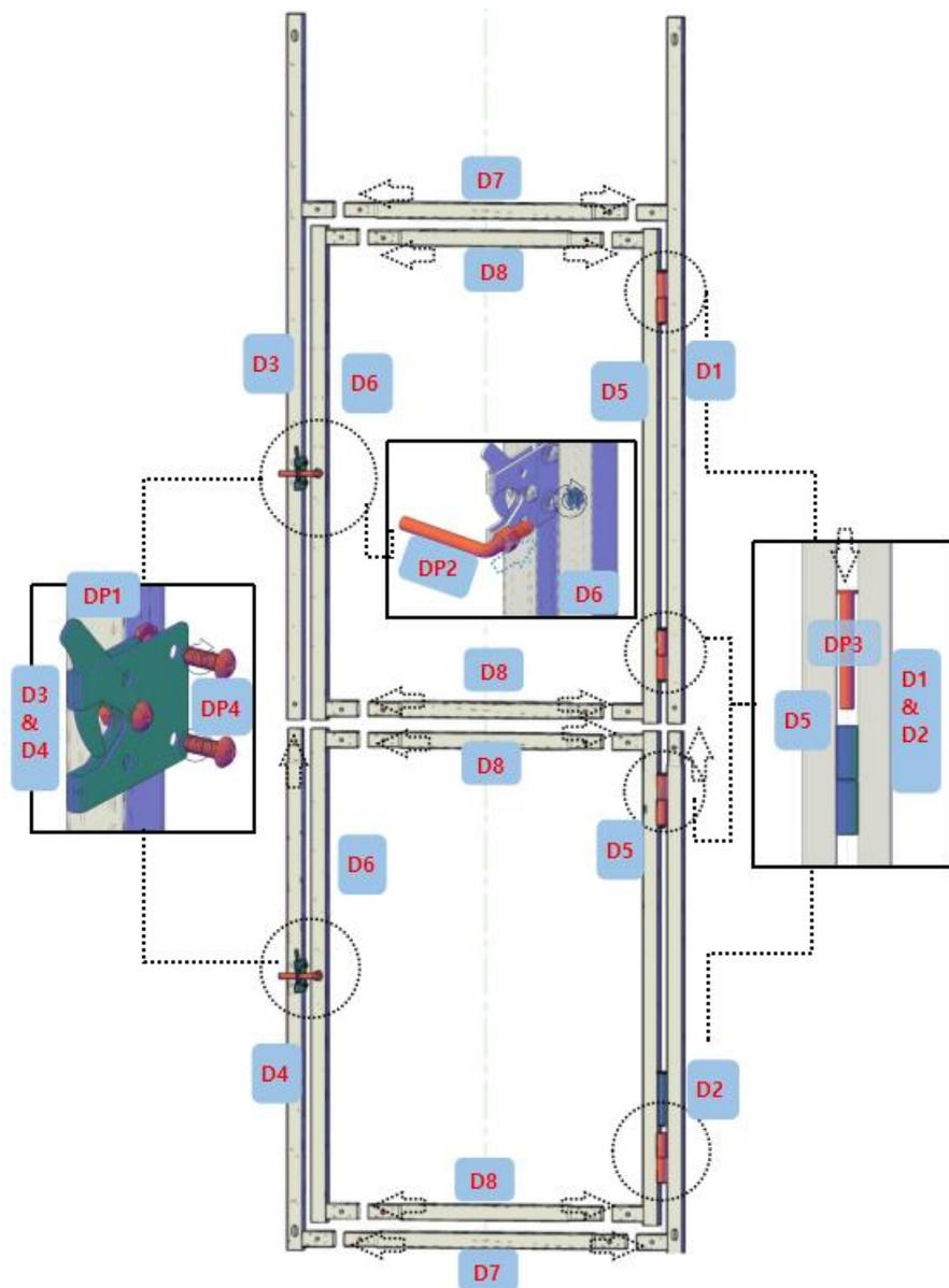
**Step7:** Attach the door to the frame.
