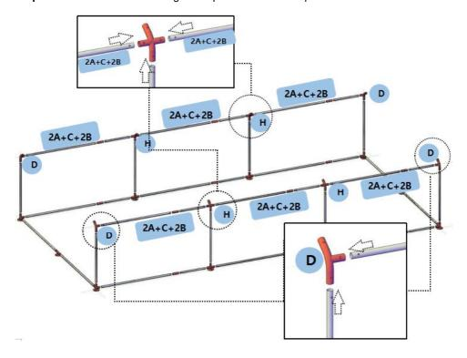
**Step5:** Install the top surface according to the part number in the figure below.
