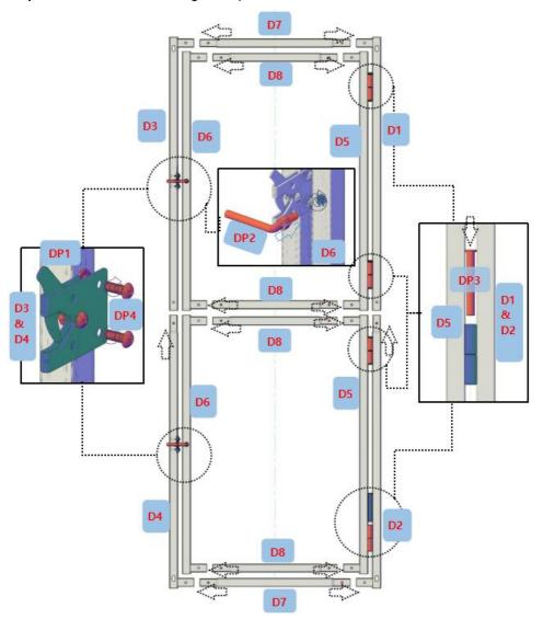
**Step7:** Attach the door to the frame.
