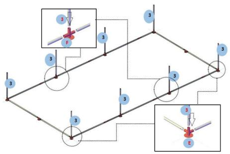
**Step4:** Install the beam according to the part number in the picture below.
