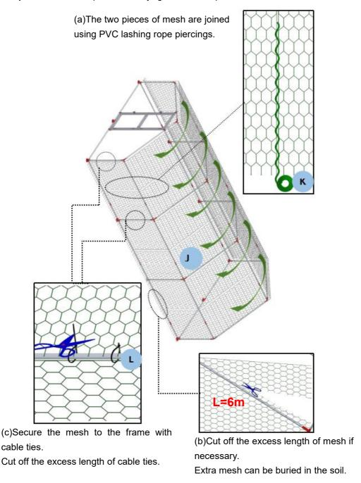
**Step9:**Install front and rear mesh (The two mesh are interlaced with PVC lashing rope) and secure to the frame with excess length cut.
