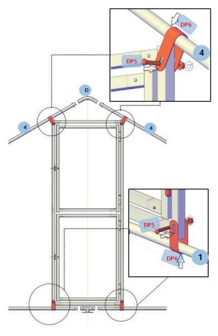
**Step8:** Installation of top mesh. The laying mesh can be pre-cut to 6x1m.
