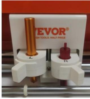
2. Place the Blade and housing in Clamp R. Place the pen or the foil transfer and housing in Clamp L.
