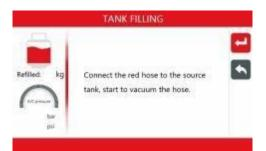
11) Tank filling completed.Press **back** to MAIN MENU. Select another type of refrigerant for TANK FILLING.
