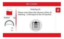
8)) Recovery completed. Check the recovery amount and oil drain amount. Touch to print or exit.
