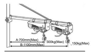
Location A: Load capacity: Max300kg , Arm: Max 700mm; Suitable for 2200lbs Electric Hoist Location B: Load capacity: Max150kg , Arm: Max 1100m; Suitable for 440lbs-1800lbs Electric Hoist
