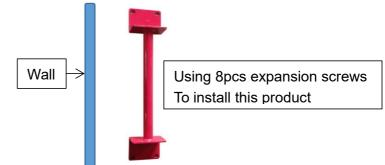
Step 2- Install the "locking casting".
