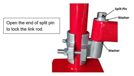
**Step 5**- Insert the link into the pin on the top locking casting, and then install the split pin. After installing the split pin, make sure to open the end of the pin to confirm that the split pin cannot fall out of the locking pin hole.
