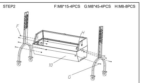
Fix the support foot and grill body with M8\*45, M8\*15 hexagon screws and M8 flange nuts.
