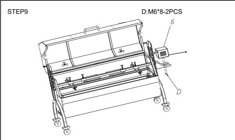
Put the motor on the motor support plate, and lock it with M6\*8 hexagon screw. Put the slag plate on the bottom slot of the grill body. The installation is complete.
