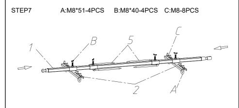
Fix the food in the proper position of the barbecue fork as shown above, and use M8 \* 40 to lock the positioning plate and the baking fork with dished screws, then lock the U-shaped bolts passing through the positioning plate with M8 butterfly nuts.
