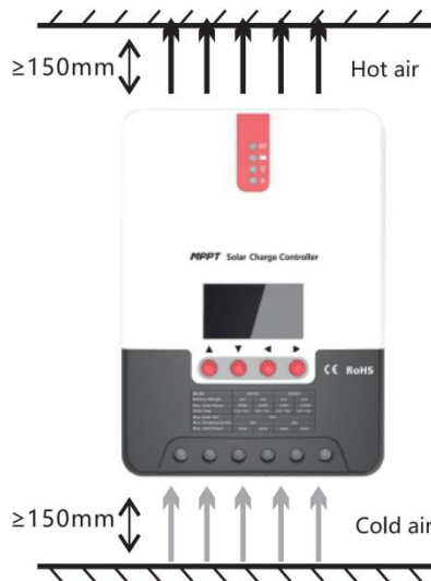
Fig. 2.1 Installation and heat dissipation
